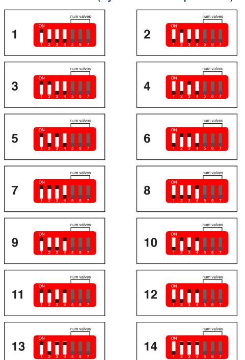
Drone Valve Outputs (all Drones should have the same number of valves)
